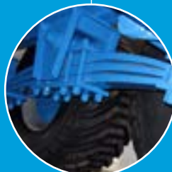
High Quality ADR Suspension System (Tandem and Tridem axle models) reduces jolts and impacts travelling through to the tank. Hydraulic or Air suspension also available. Providing greater stability and operator safety.
