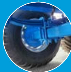
High Quality ADR Suspension System (Tandem and Tridem axle models) reduces jolts and impacts travelling through to the tank. Hydraulic or Air suspension also available. Providing greater stability and operator safety.
