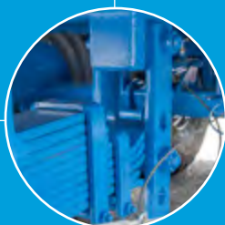
Pre-Tensioned Drawbar Suspension For smoother travelling
