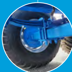
High Quality ADR Suspension System (Tandem and Triple axle models) reduces jolts and impacts travelling through to the tank. Hydraulic or Air suspension also available. Providing greater stability and operator safety.
