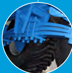
High Quality ADR Suspension System (Tandem and Triple axle models) reduces jolts and impacts travelling through to the tank. Hydraulic or Air suspension also available. Providing greater stability and operator safety.
